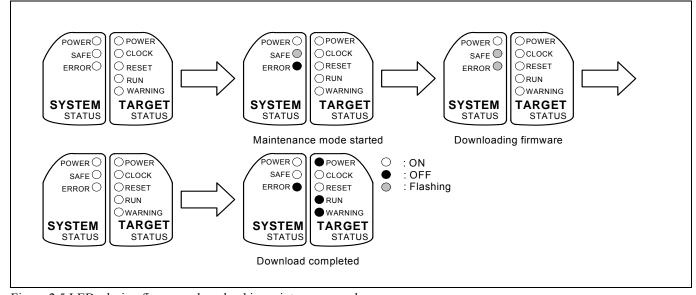
Figure 2.5 LEDs during firmware download in maintenance mode
